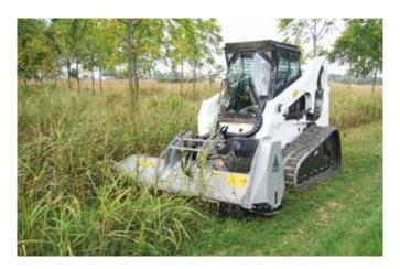
Attachment plate with self levelling device Self levelling protection rubber Possibillity to have the rotor equipped with PML hammers or Y-flails
