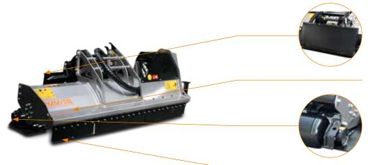
Attachment plate with self leveling device adapts to all types of terrain
